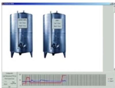
SCADA - SPR8 System supports centralised computer aided operation of SPR8 controllers from a central location. Up to 247 temperature controllers SPR8 can be linked in a network and controlled respectively. This clear and easy to use program is an efficient solution for wine
