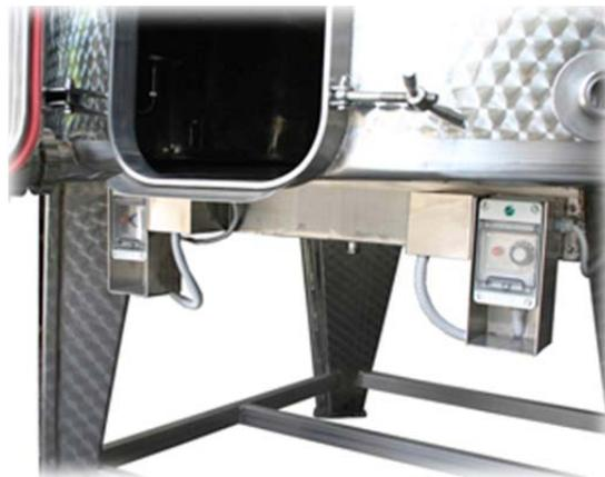
The double bottom is a specially designed bottom of the vessel with a water reservoir and electric heating elements. The heating function may be controlled either manually with a thermostat on the heater, or automatically (heater on/off) by means of a SPR8 temperature controller.
