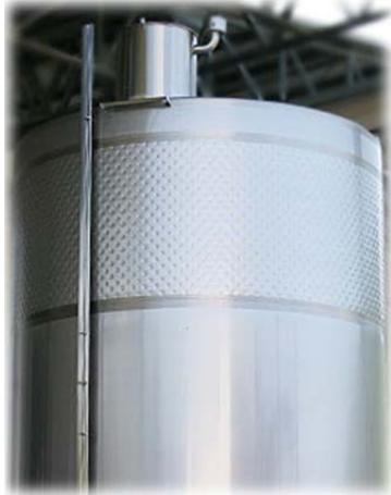
The double jacket is a component of the vessel envelope, designed to allow the control of temperature in the vessel by adjusting the through-flow of cooling/heating medium. Corrugated external sheet and the vessel envelope form an enclosure for the flow of the cooling/heating medium.
